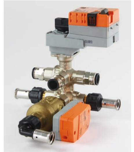
Pressure-independent assembly for a heating/cooling ceiling sail consisting of a 6-way characterised control valve and a PIQCV. Equipped with press connectors and quick couplings.
