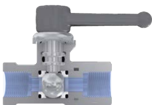
Valve open position
