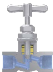
Valve open position
